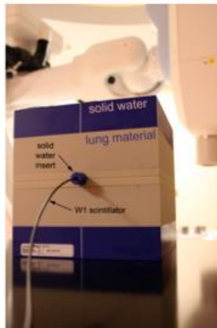
Fig. 2 – components of lung material phantom
