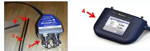
Figure 1. W1 elements: (1) scintillator detector, (2) optic fiber, (3) Photo-detector, (4) 2 channel electrometer.
