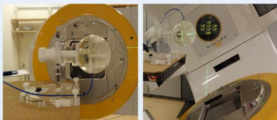
Figure 3. DD inserted in Lucy phantom for measurements: left tip up, right tip down.
