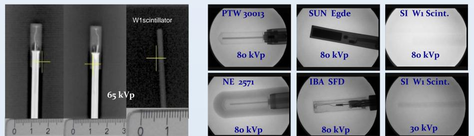
Figures 4. (a-b) DD orthogonal views (65 kVp) in air, (c) W1 view (65 kVp) in air, (d) ionization chambers and W1 view (80kVp) in water. W1 is visible only with 30kVp X-ray.
