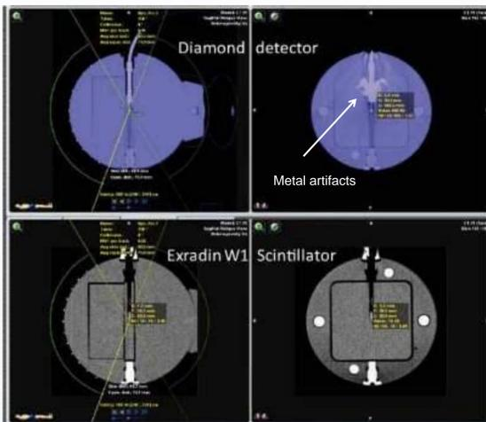
Figure 2. In blue the Lucy phantom with the DD and in grey, bottom, with the PSD, position "tip down".
