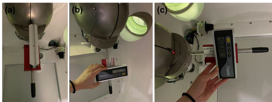
FIGURE 8 (a) Home, (b) North Pole, and (c) Patient Right positions of the linac for gantry angular accuracy check. linac, linear accelerator.
