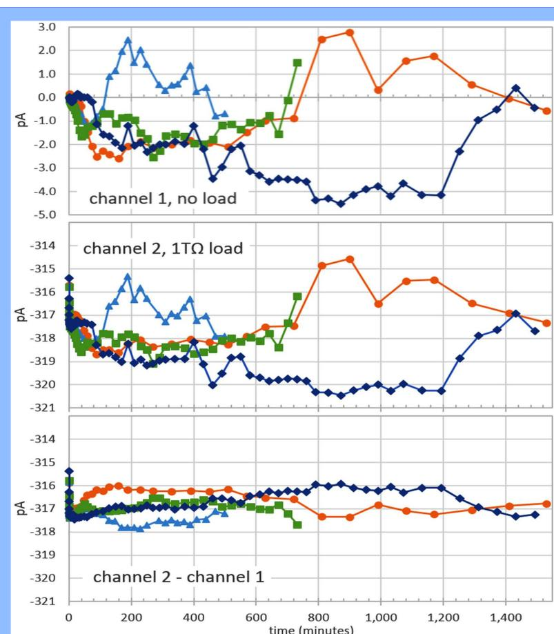
Figure 1: Electrometer operated at -300 V and connected to no load on channel 1 (top) and 1TΩ load on channel 2 (middle); both channels display very similar fluctuations, independent of load. Subtracting channel 1 from channel 2 reduces the fluctuations and current remains constant within  $\pm 1$  pA over up to 25 hrs (bottom).
